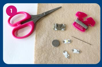
Prepare your work space, we recommend using the E-Textiles Starter Kit, as it contains all of the electrical components you will need. Start by threading up a needle with the conductive thread, you may need to use a needle threader for this. Line up your cell battery and sewable LEDs to cover the area you need.
