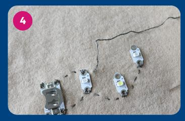
Create a knot at the end of a new piece of conductive thread and sew the next path (positives) from the cell battery to the positive loops of the sewable LEDs. At no point must the thread pathways meet or cross over each other from the positive and negatives.
