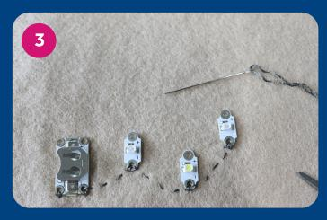
Sew to the end of your path, we have started with the negatives. Secure your thread at the back by creating a knot and trimming the end of the thread. You don't want to have any long loose threads underneath the circuit as this can affect the current.
