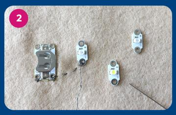
You will need to align the positive and negatives so that they match up to each other. E.g. the negative ends of the cell battery will line up with the negative ends of the sewable LEDs. Start by securing the end of the conductive thread with a knot, and sewing from loop to loop in the positions needed.
