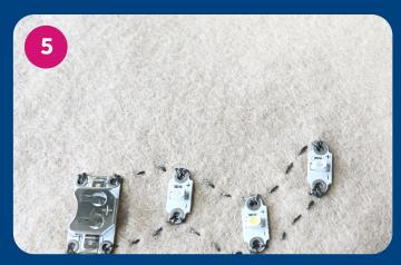
Once this path is completed, secure the end of the thread underneath your fabric and trim. Your circuit should now be complete. Carefully place the coin cell battery into the slot in the cell battery, the postive side upwards. Your LED lights should be lit up!
