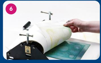
Place a piece of Newsprint on your press, and lay your etched plate face-up, on top of this. Use runners along the full length of the printing press on either side of the plate. Carefully lay a piece of damp paper on top. Cover with another piece of newsprint and the press blanket. Roll print, then remove with clean fingers and leave to dry thoroughly.
